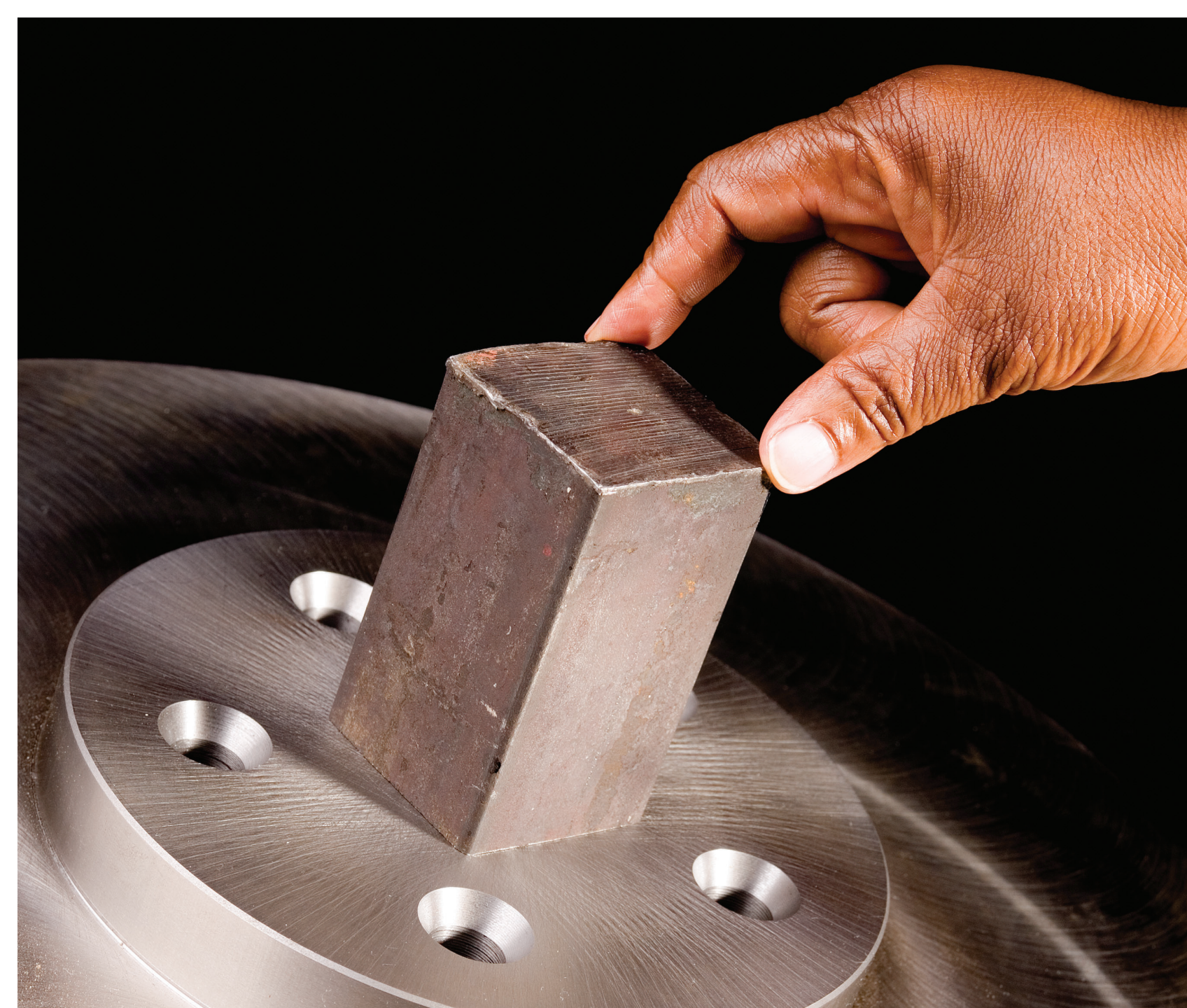
Picture 3: A VCI-protected metal item (without corrosion) and an unprotected, corroded metal item
