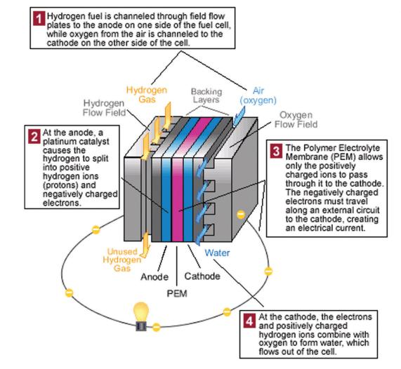
According to a dictionary definition, "A Fuel Cell is an electrochemical cell in which the energy of a reaction between a fuel, such as hydrogen, and an oxidant, such as oxygen, is converted directly and continuously into electrical energy."
