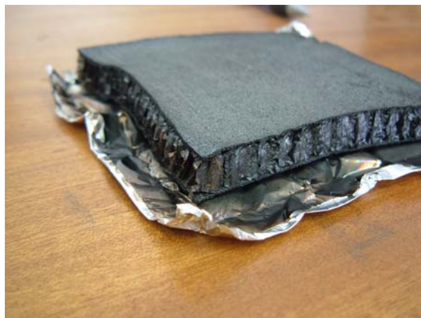
Figure 5: Composite panel after testing in the cone calorimeter. Note charring of all layers.
