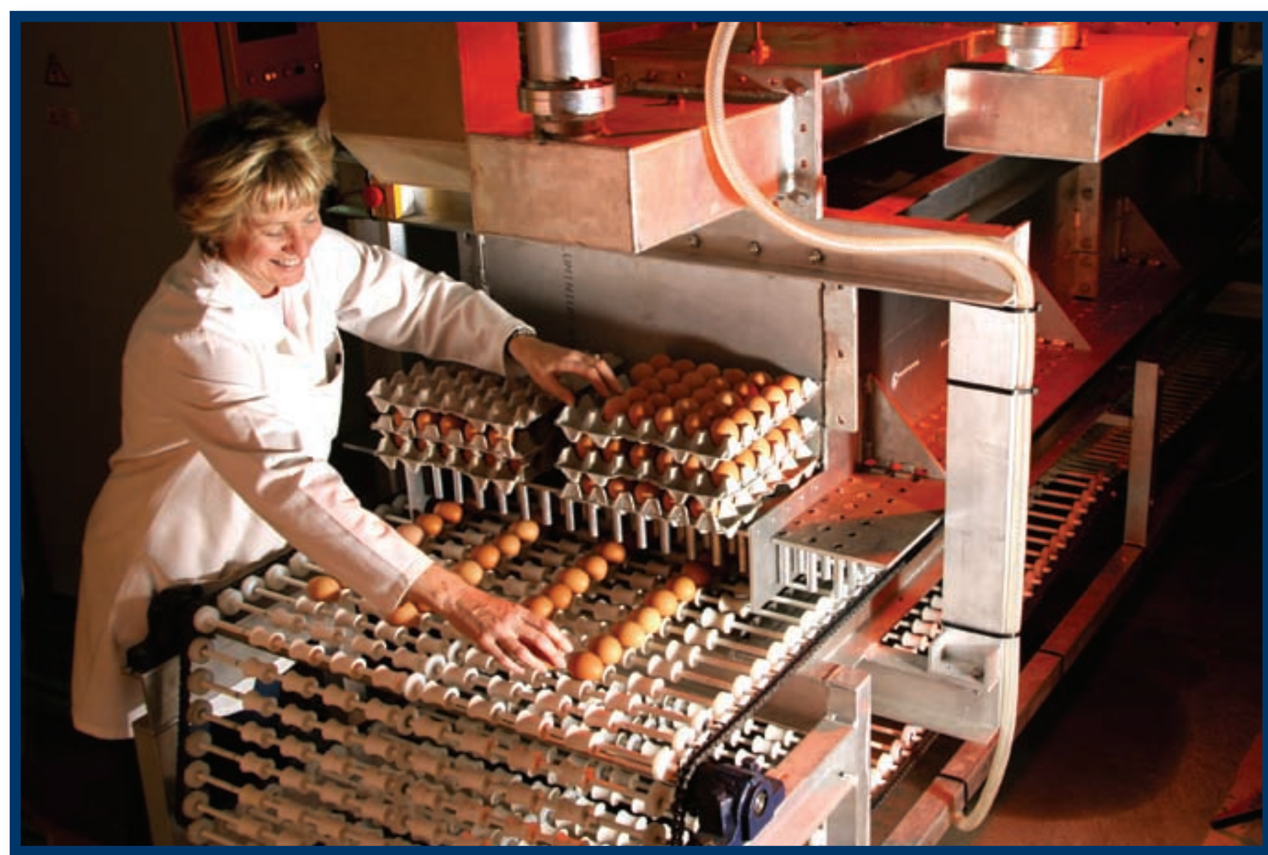
Figure 1. Loading of the rolling bed with eggs going into the microwave cavity of the pasteuriser
