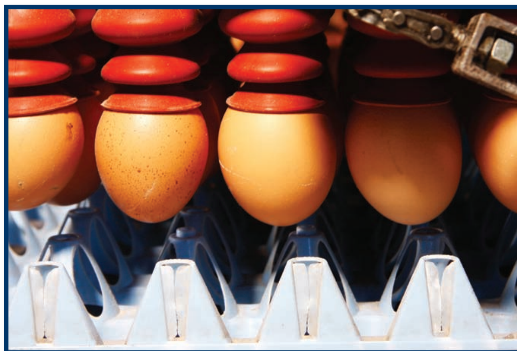
Figure 1. Loading of the rolling bed with eggs going into the microwave cavity of the pasteuriser
