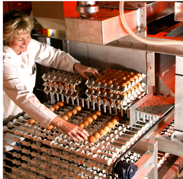
Figure 1: Loading of the rolling bed with eggs going into the microwave cavity of the pasteuriser.
