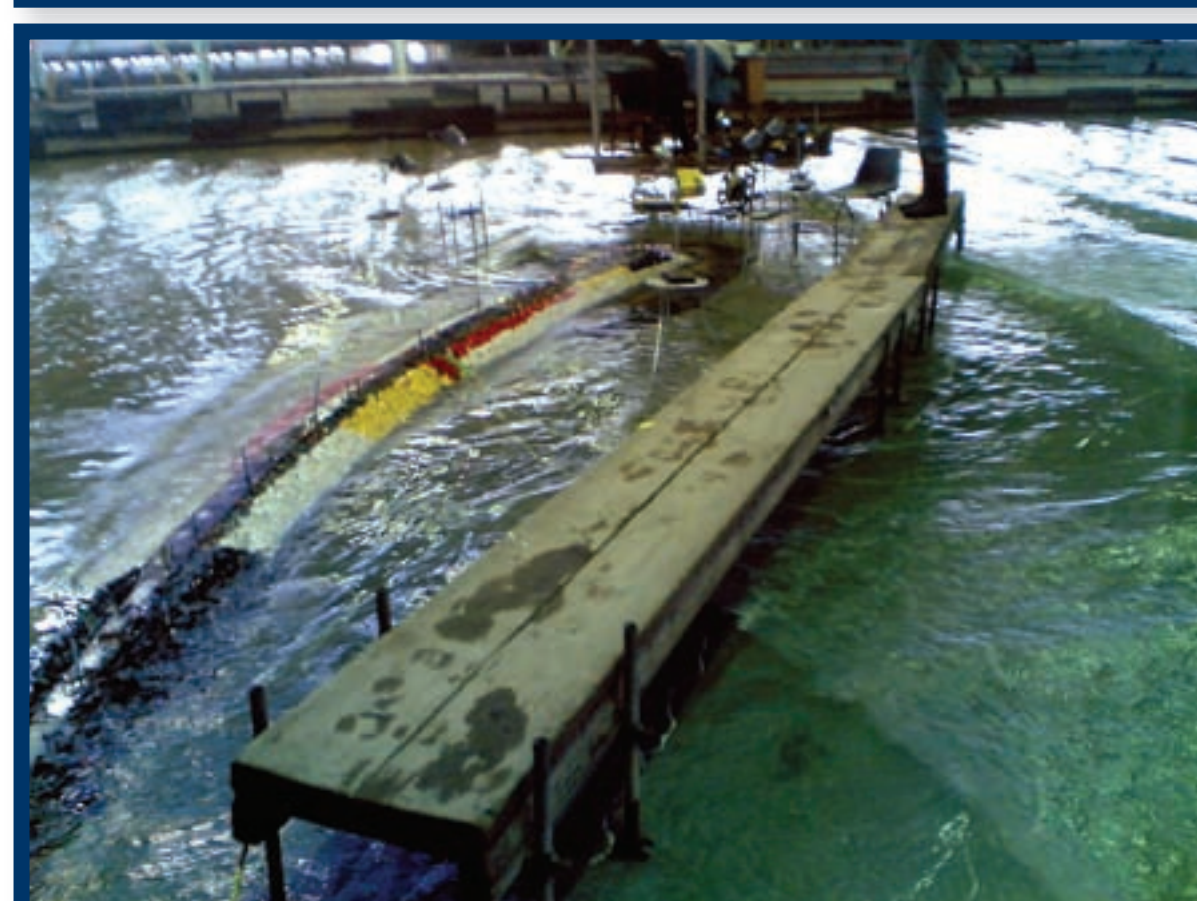
Figure 5: A view of an experiment in progress with generated waves interacting with the model breakwater structure under study. The wave generators are to the right of the photograph. The instrumentation set up around the model records the characteristics of the waves during the run. Changes in the physical model are recorded using photography.
