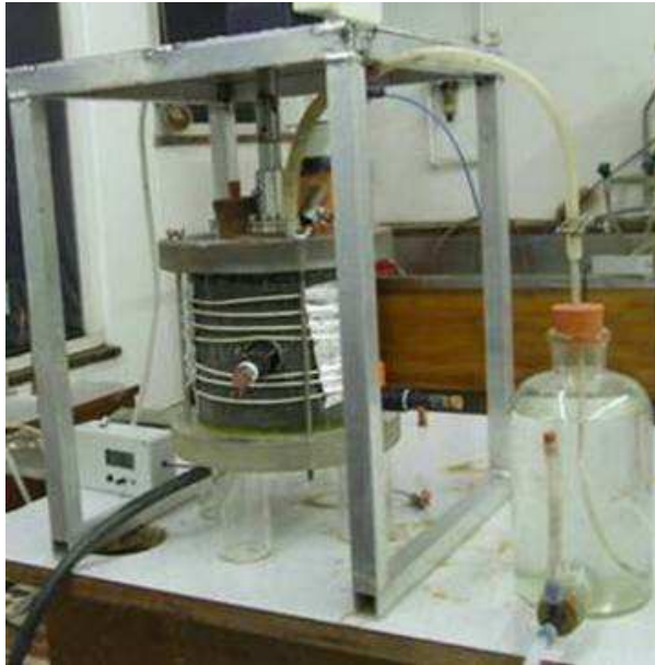
Figure 1. Laboratory Scale Anaerobic Digester (AR)
