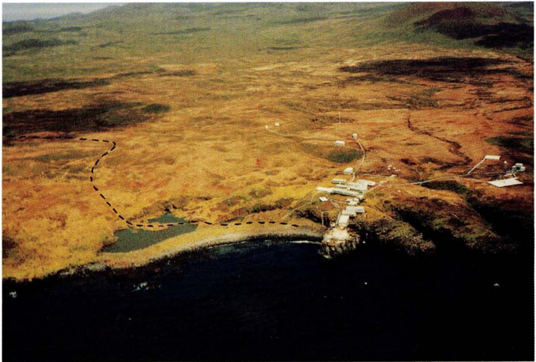
FIGURE 5.2 Oblique aerial photograph of Transvaal Cove. The Base Station extends seawards along Gunners' Point, which provides a shelter to the northern end of the boulder beach. A channel will be cut through the kelp bed in the deeper waters of the Cove, to give access to a landing ramp to be built on the northern end of the beach. The road to the ELS follows the route marked in black.
