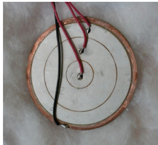
Fig. 2: Prototype deformable mirror (rear view).
