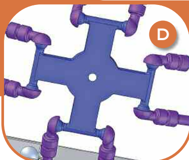
Figure 1 a. All movable parts of 4-armed PKM machine b. Bottom view c. Lower leg components illustrating 'knee' and 'ankle' joints d. Close-up view of the robot hand (end-effector)
