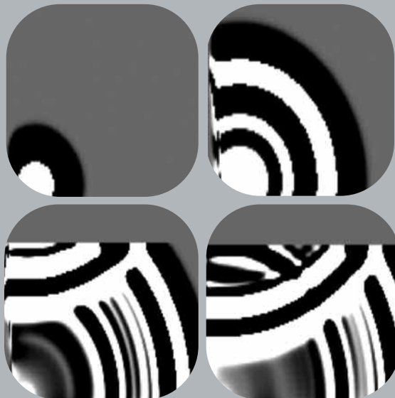
Figure 6 Snapshots of electromagnetic waves propagating from the transmit antenna to the receive antennas
