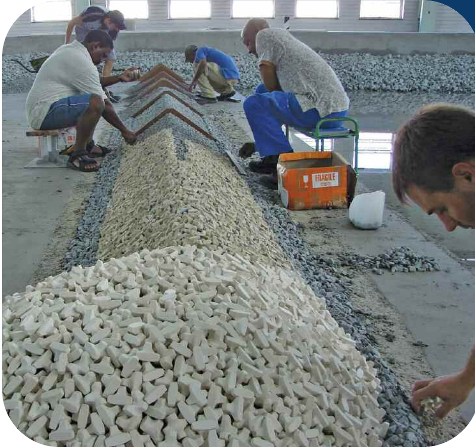
Khalifa Port's main breakwater model under construction in the CSIR's hydraulics laboratory in Stellenbosch
