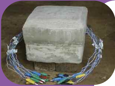
The 1:400 cement model is a scaled equivalent of the 3D mining layout and geophysical sensor configuration depicted in the schematics shown to the right
