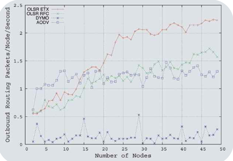
Typical graphs that can be generated by the wireless grid: This graph compares the number of outbound routing overhead packets per node per second as the number of nodes increases for four different routing protocols. Routing overhead needs to be minimised as it uses up valuable capacity in the network that needs to be used to send data over the network
