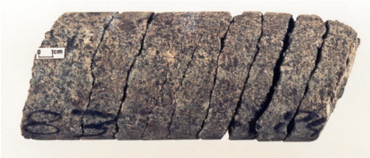
Figure 10 Non-symmetrical core discing, indicating that the core axis is not a principal stress direction
