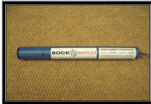
Figure 2.3.1 The modified transducer in a plastic housing.
