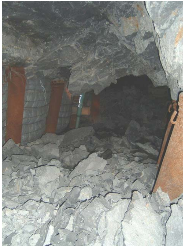
Figure 4.2.4 Fall of ground in the E8 panel next to the 0302 closure meter (looking down dip).
