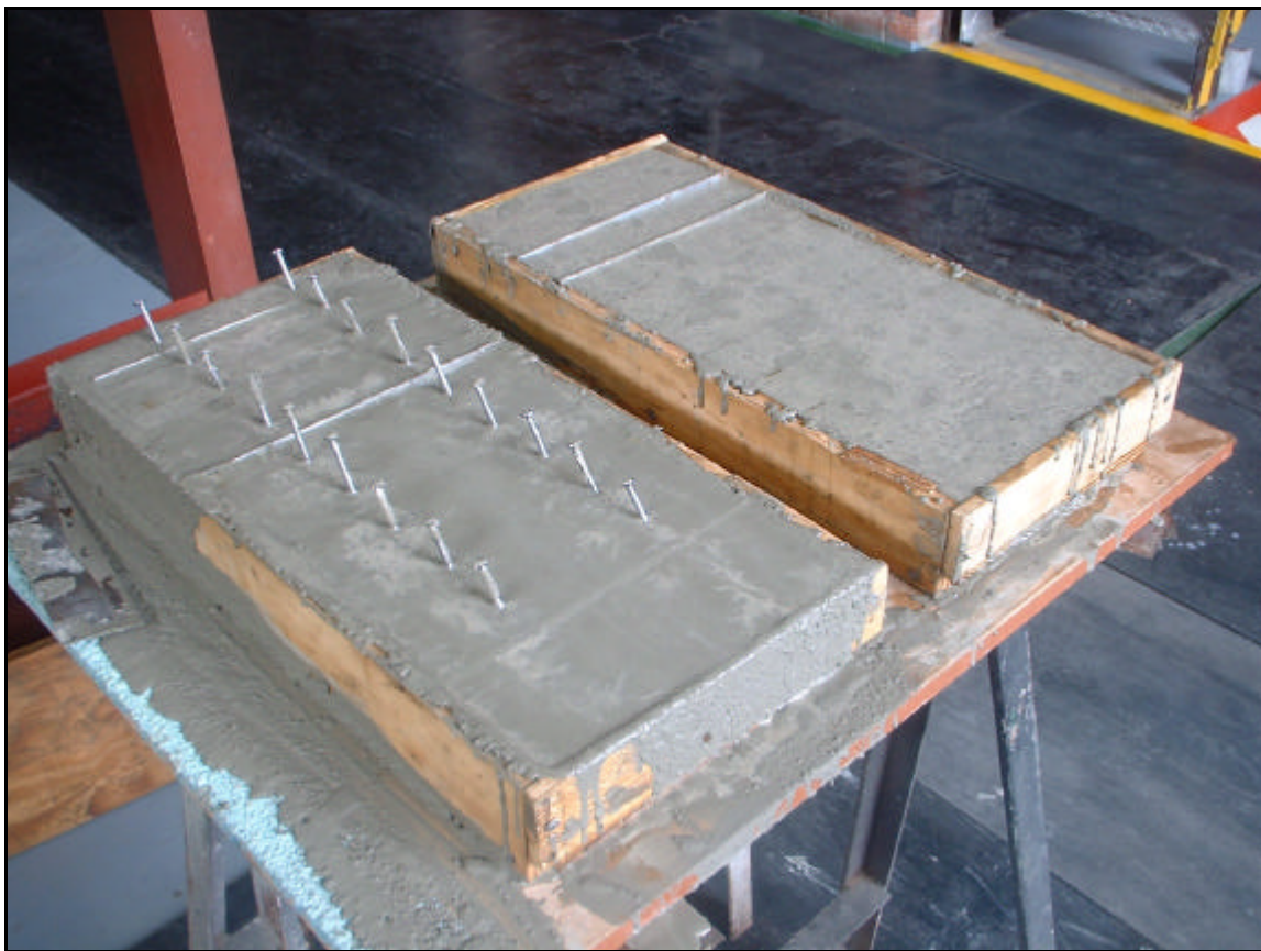
Figure 22. Tray moulds for unbolted and bolted layers after concrete pouring
