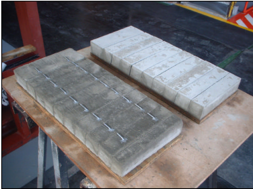
Figure 24. Lower bolted layer and upper unbolted layer
