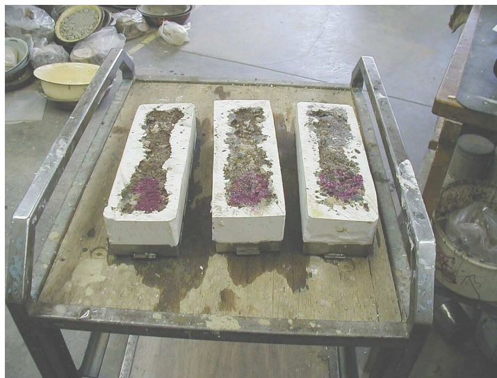
Photograph 6: Site cured beam (56 compaction hammer blows), site cured beam (42 compaction hammer blows) and humidity room cured beam prior to erosion beam test showing the dark pink colour stain of the phenolphthalein solution (Semmelink et al, 2002)
