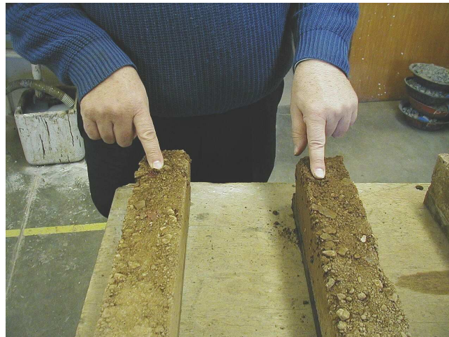
Figure 5: A similar loose layer formed in the top layer of the two samples. This is the water simulated process without the presence of CO 2 done in the laboratory (Semmelink et al, 2002)
