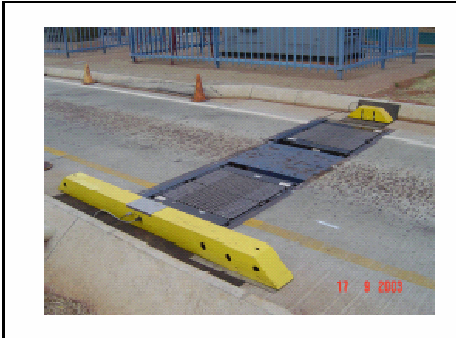
Figure 1: In-situ configuration of the SIM Mk IV (4 pads) system ready for testing at N3-TCC
