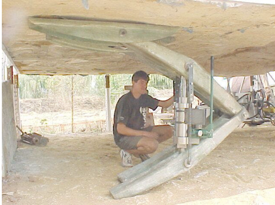
Figure 5-4: Photo of roof support system in mock-up stope.
