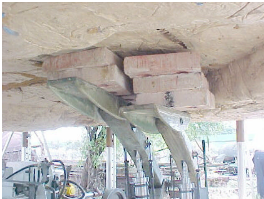
Figure 5-4: Photo of roof support system in mock-up stope.
