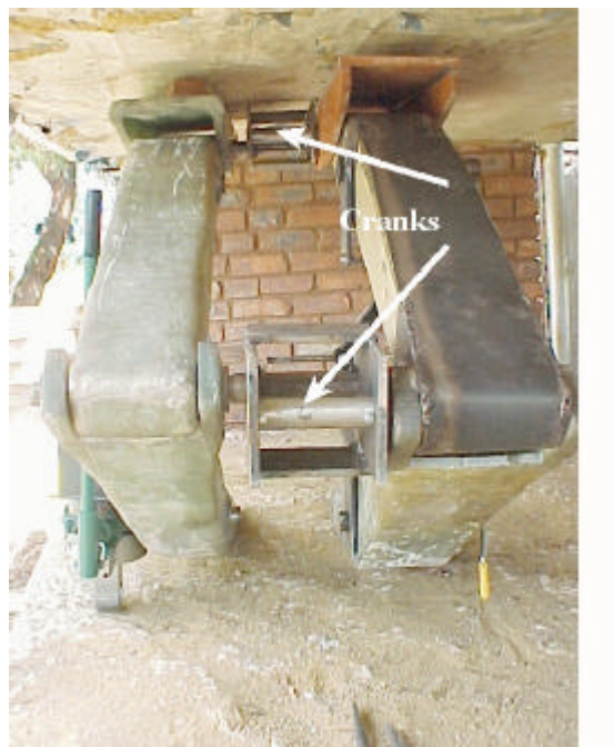
Figure 4-14: Photo of connecting crank for parallelogram of walking mechanism.
