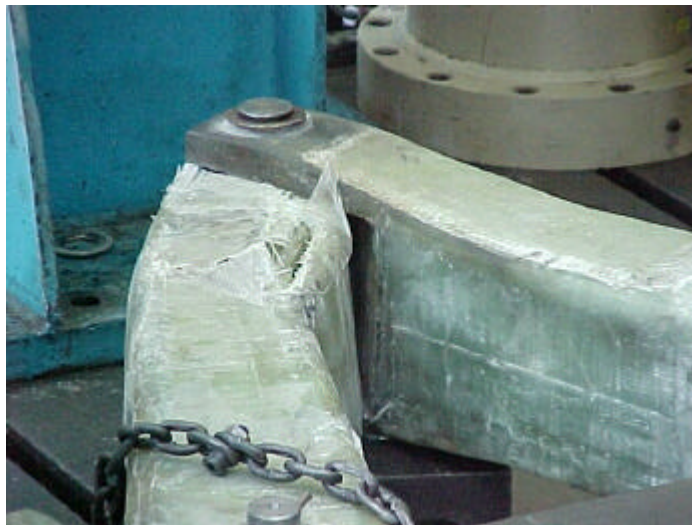
Figure 5-2: Photos of damaged top leg of wishbone.
