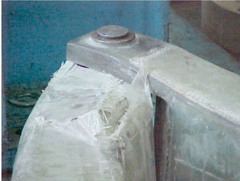
Figure 4-17: Failure of top leg in hinge area.
