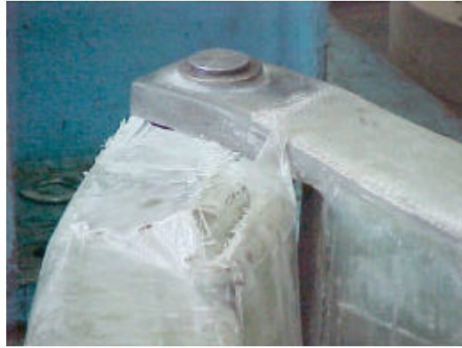
Figure 4-7. Failure of top leg during testing.
