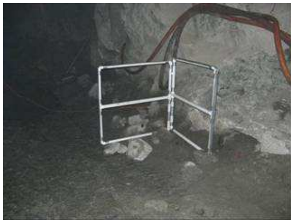
Figure 2: Orthogonal 1 m x 1 m receiver coils as used underground for noise recording.
