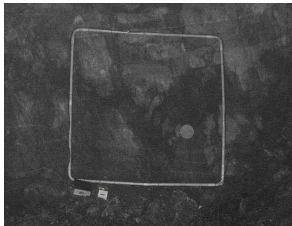
Figure 1: 3m x 3m Tx/Rx coil deployed underground against the mining face.
