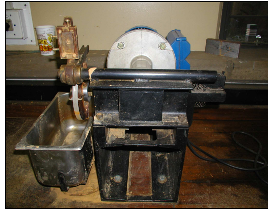
Fig 1. Abrasive wear testing device with rotating wheel.
