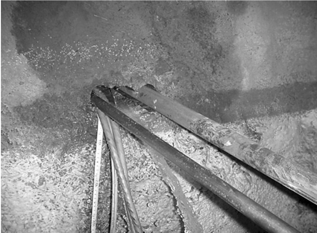
Figure 5.2.5 Photograph of drilling of third borehole past the measuring device during testing at Impala Platinum mine
