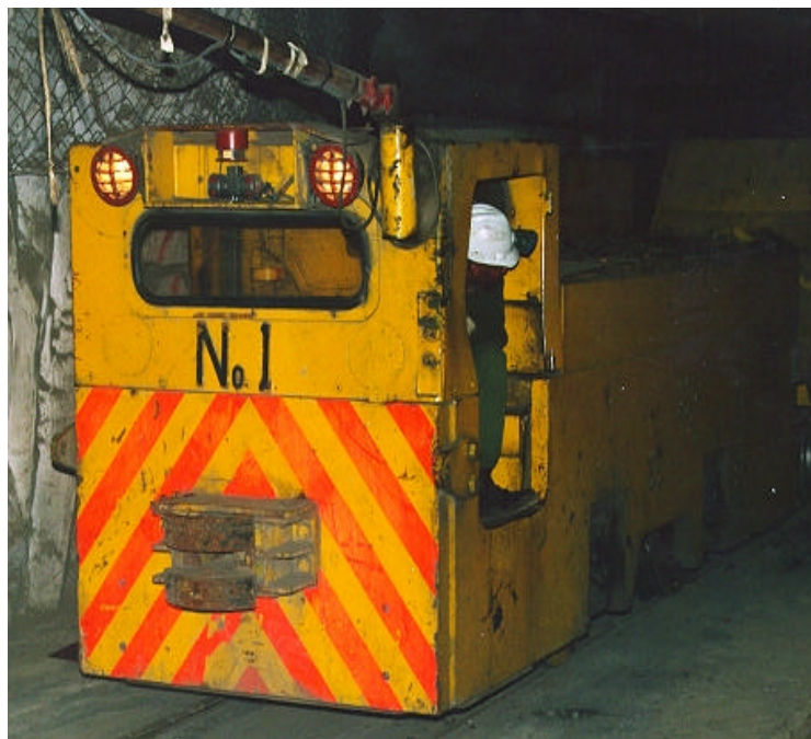
Figure 4.2.6.2: Electrical locomotive with enclosed cab
