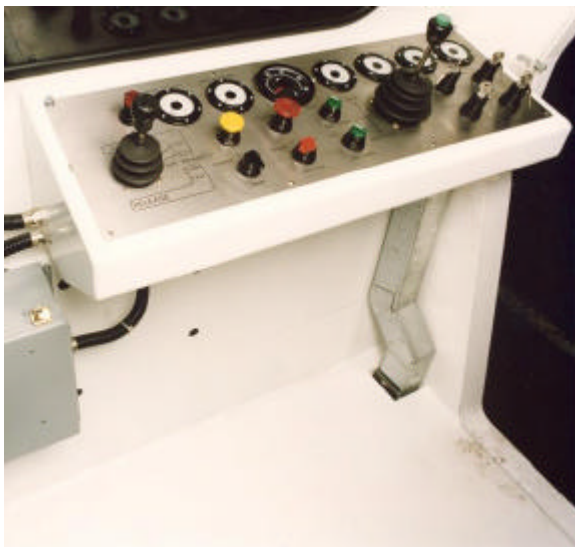
Figure 1.5.1: Trolley control panel (Europe)
