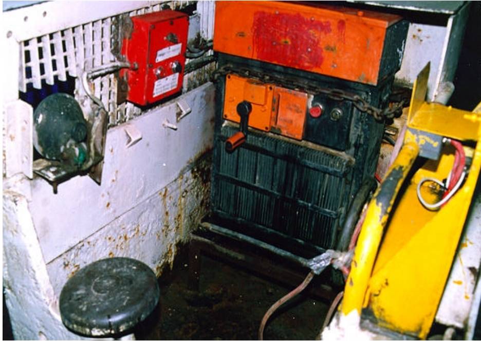
Figure 4.2.8.2: Control layout with master controller opposite seat
