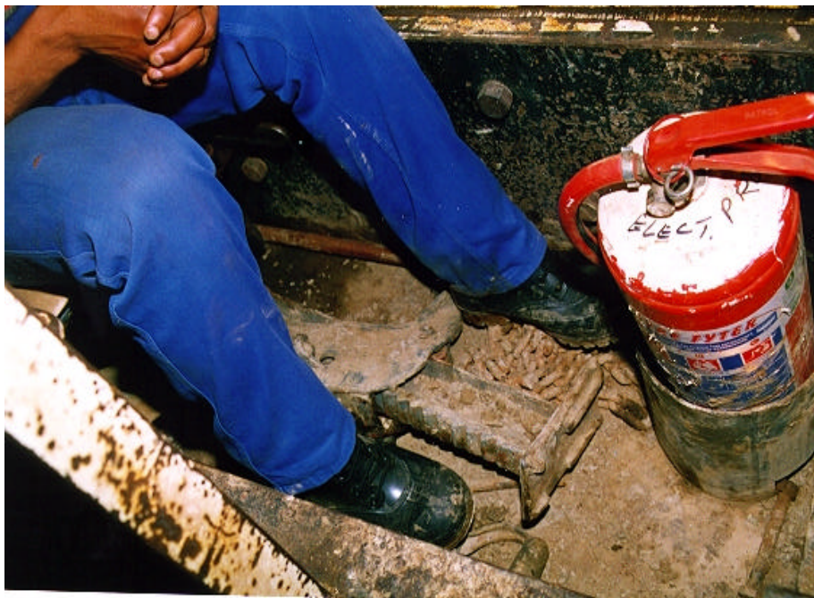
Figure 4.2.3.1: Jack, chain and other equipment encroaching on foot support and space
