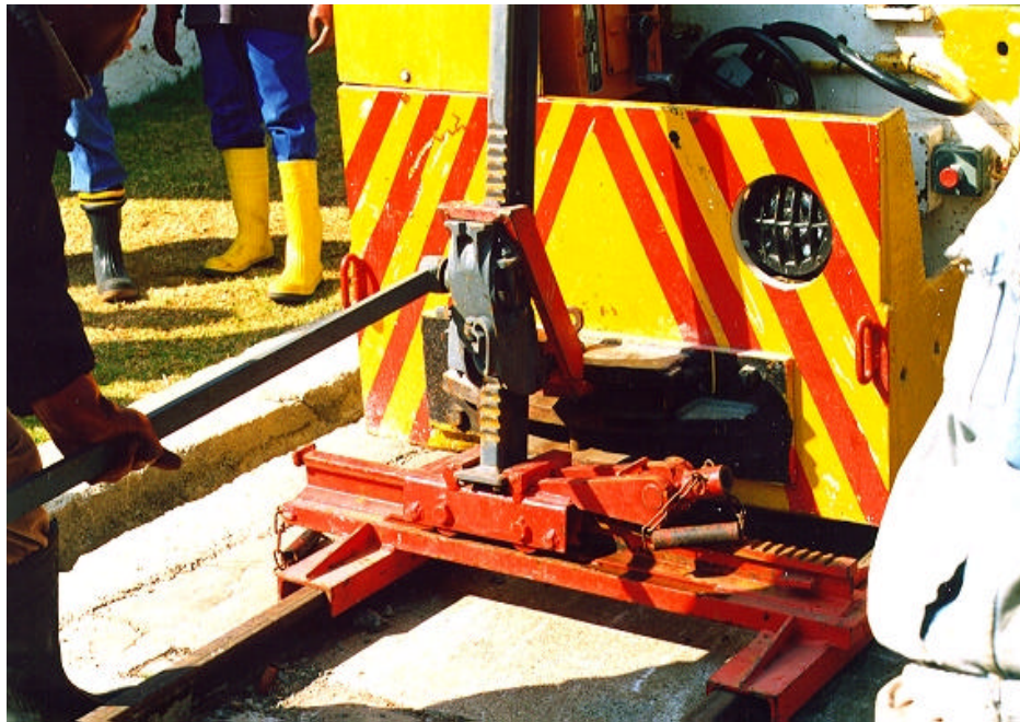
Figure 4.2.9.2: A mechanically assistive re-railing device
