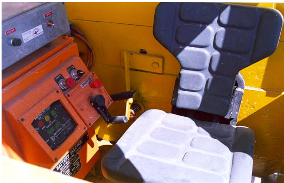
Figure 3.2.2.2: T-shape backrest with horizontal adjustability
