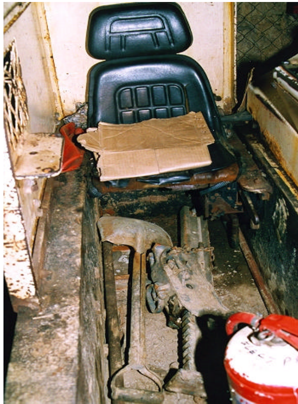
Figure 2.3.3.3: Worn seat base
