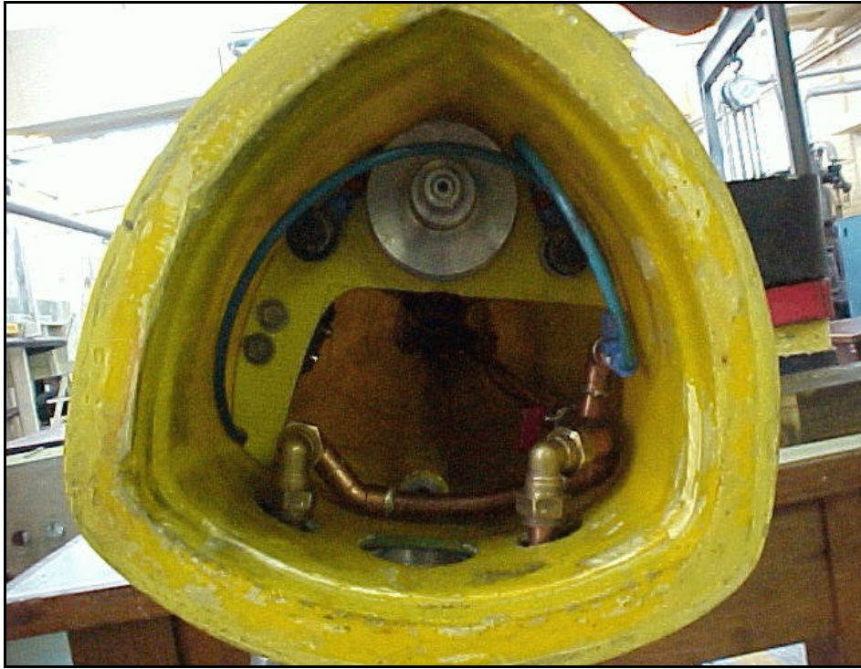
Figure 6-2 Inside of tube of quiet rock drill (XDM)
