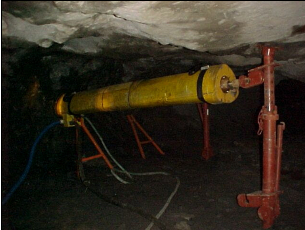
Figure 9-3 Photo of quiet rock drill being tested underground
