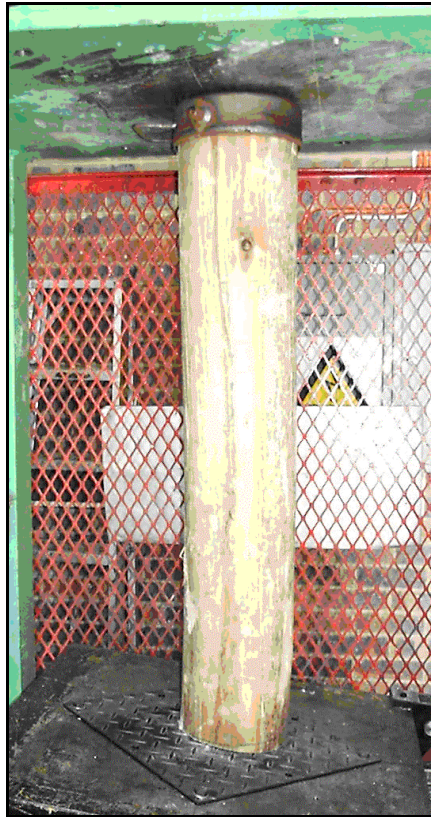
Figure 4.3.8 Photograph showing the test set-up for the slow deformation rate tests.
