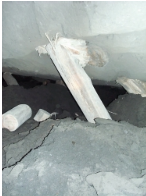
Figure 2.3.6 Photograph showing oblique and rotational loading of elongates.
