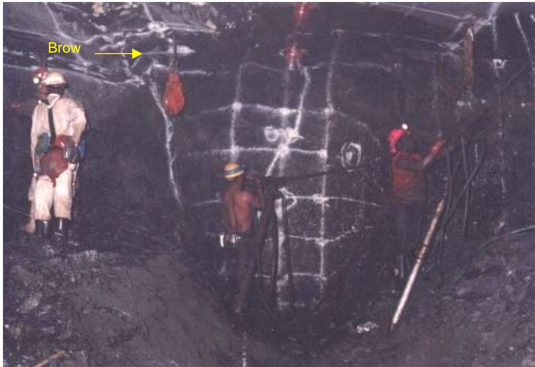
Figure 4.43 – Development-type round with a burn cut, used to advance an ASG-type gully, here shown in a high stope width area at shallow depth
