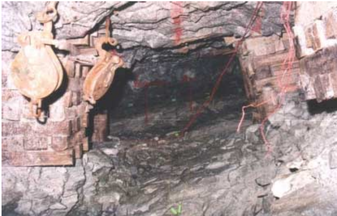
Figure 4.43 – Development-type round with a burn cut, used to advance an ASG-type gully, here shown in a high stope width area at shallow depth
