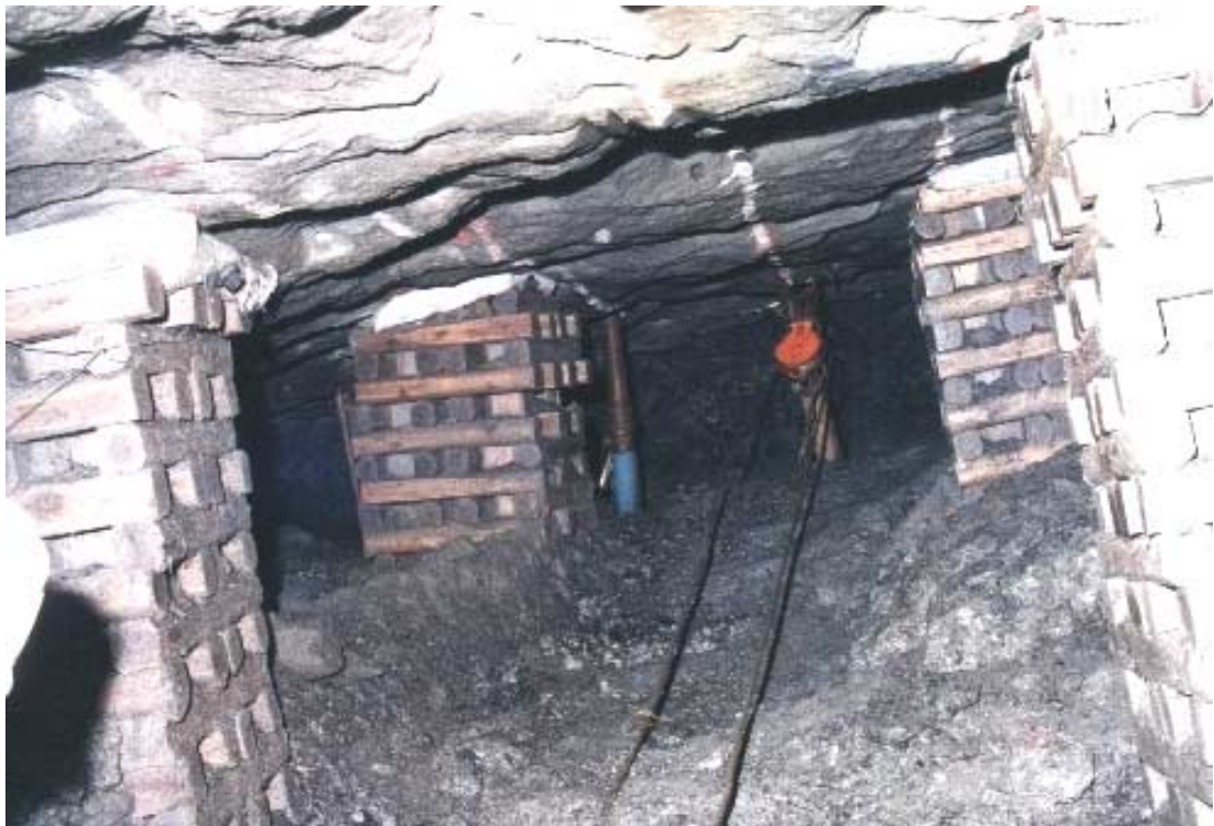
Figure 4.23 - Merensky Reef - conditions in a wide heading with footwall lifted gully at 2000m below surface
