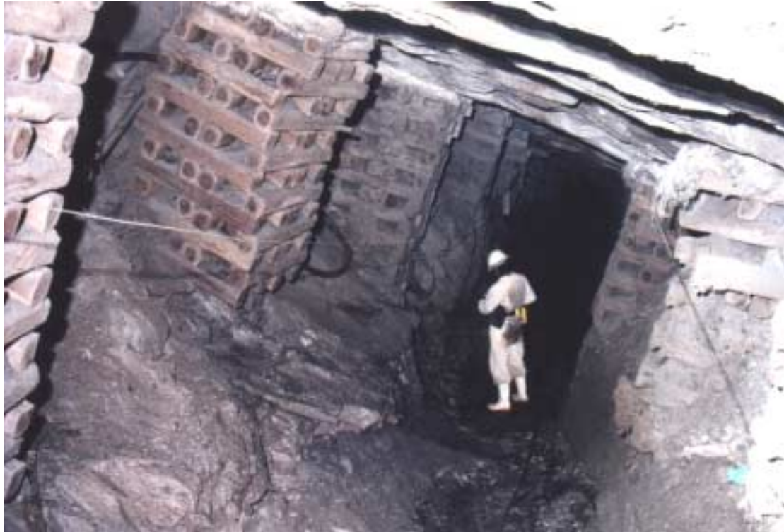
Figure 4.22 – Merensky Reef - footwall lifted gully in wide heading at 2000m below surface. Due to down dip sidewall integrity, all packs are normal to dip
