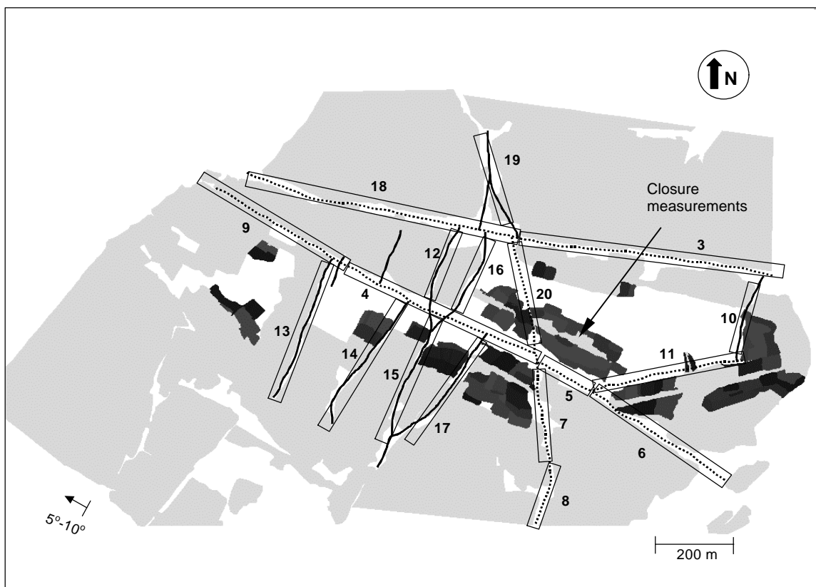
Figure 31 The Vaal Reefs No. 5 shaft region that was modelled. In this plan all major geological discontinuities are shown (enclosed in numbered rectangles). The extent of mining that occurred prior to the analysis start date is shown as grey and the recent mining is indicated in darker shades of grey. The stope where rock mass displacements were recorded is also indicated.
