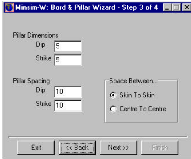
Figure 6-3: The third window of the MINSIM Bord and Pillar Wizard dealing only with parameters actually relating to the pillars.
