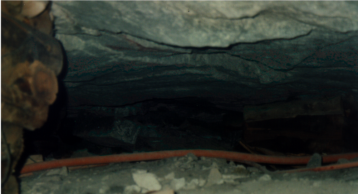
Figure A4.4.6.1 Photograph of a Carbon Leader stope showing the variation in the hangingwall parting plane amplitude
