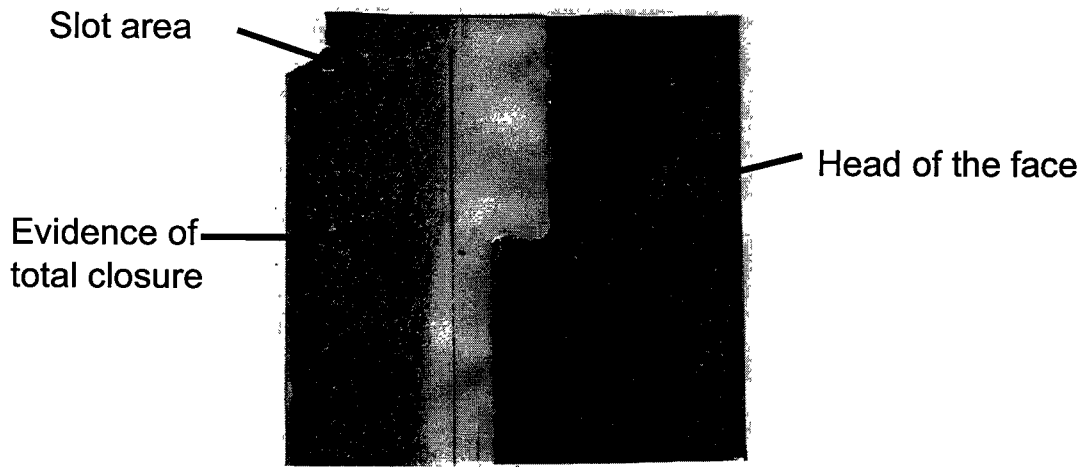
Figure A4.3.17 Stress distribution obtained from the pressure film at the interface.
