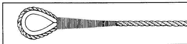
Figure 15 Spliced Thimble Termination
