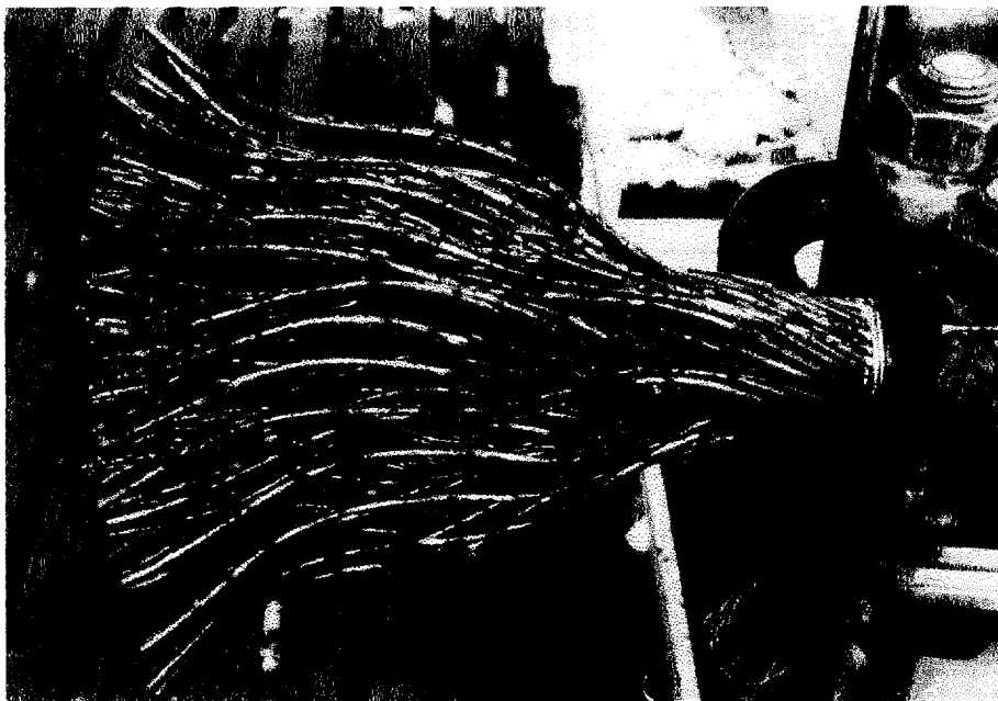
Figure 4: A photograph of the uncleaned, brushed end of the test specimen.
