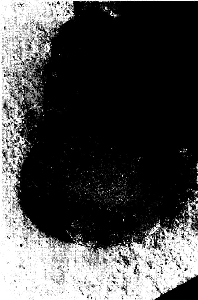
Fig. 16. Fracture surface after cleaning, showing distinct beach markings.
