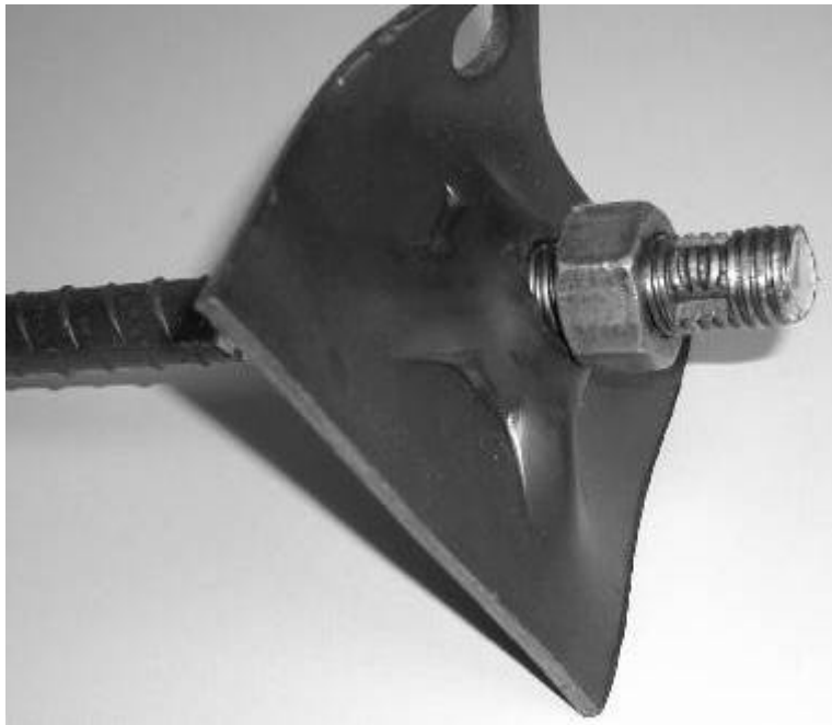
Figure 7: Standard roof-bolt stub found in Brandspruit #2. The length of stub protruding beyond the nut is approximately 30mm. Many of these bolts are installed in a mining area, and are thus perfect for connecting the seismic sensor to, providing no detailed waveform analysis is required.
