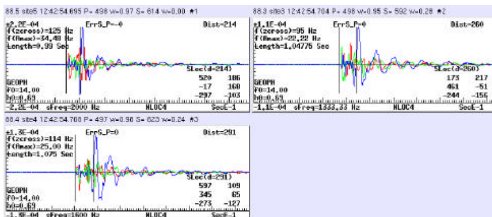
Figure 4: Tri-axial waveforms of a typical 3-station seismic event recorded by the seismic network. These waveforms exhibit clear P- and S-wave arrivals, with strong signal-to-noise ratios.
