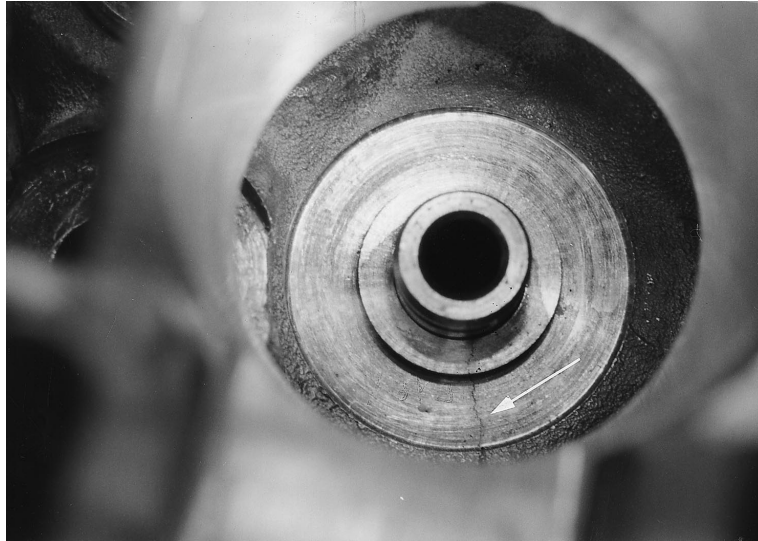
Fig. 4. The crack in the cylinder head caused by insertion of the valve guide.
