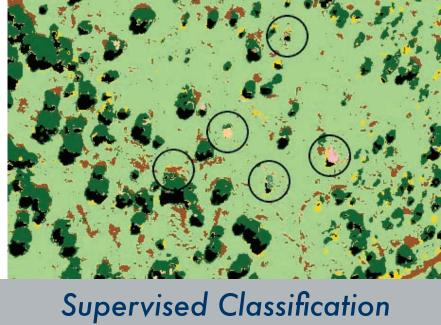
were selected as training samples. These areas was selected from the so-called "calibration site", where nets and panels, having the reflectance properties of the targets, were displayed. The software used this training data and performed an inter-comparison to the rest of the image, which contained the camouflaged objects. Supervised classification had a 63% success rate of detecting camouflaged objects.
