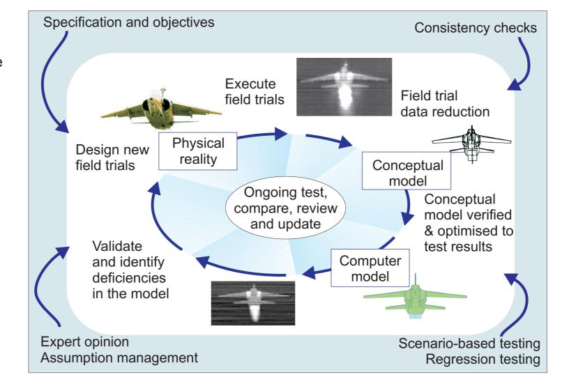
A key strength in our approach is the repeated process of measurement, data analysis, model building, software implementation and evaluation. Deficiencies in the model are detected and corrected with each iteration.
