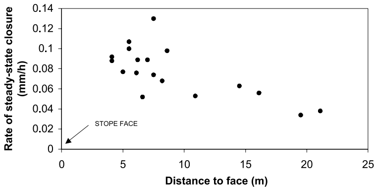
Fig. 9. Closure data from a deep tabular mining stope in South Africa. Note that the rate of steady-state closure decreases as the distance to face increases. This is contrary to what is shown by the viscoelastic model in Fig. 8. (Note that the stope face is to the left in Fig. 9 and to the right in Fig. 8.)
