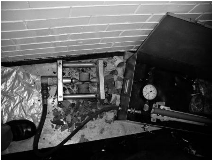
Figure 6 Arnot Colliery's Point Load Tester used to measure roof and floor cutability.
