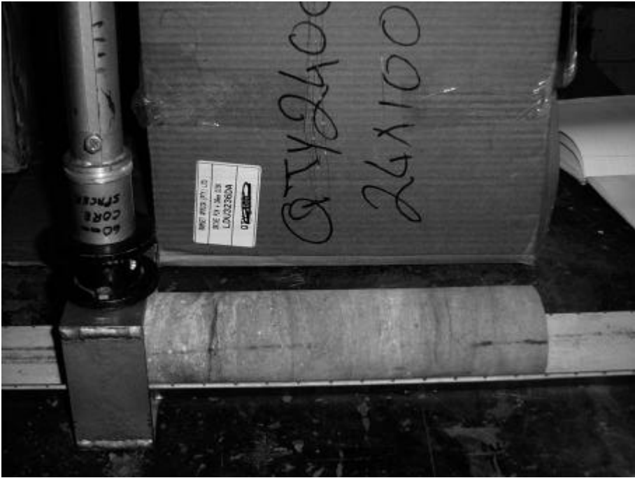
Figure 7 A fine to medium grained sandstone or “grit” unit before Impact Splitting, taken from borehole ARN 4968.
