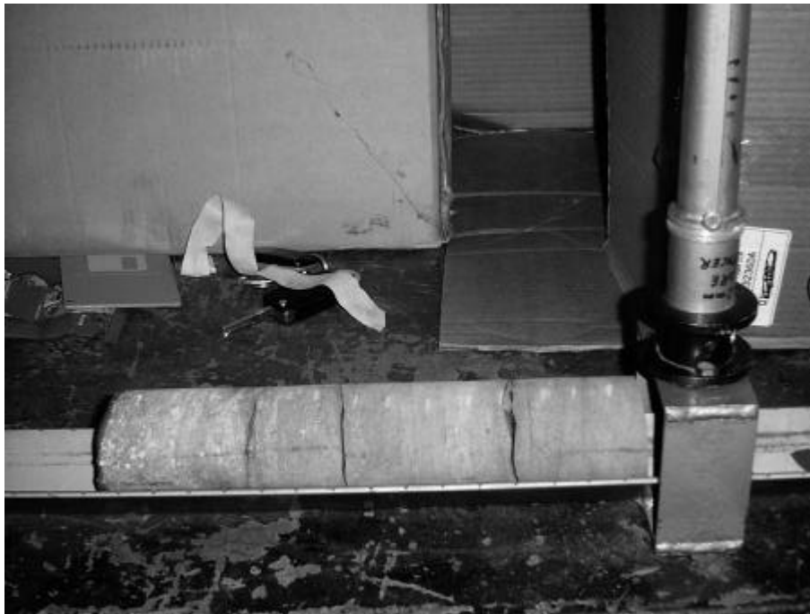
Figure 8 A fine to medium grained sandstone or “grit” unit after Impact Splitting, taken from borehole ARN 4968.
