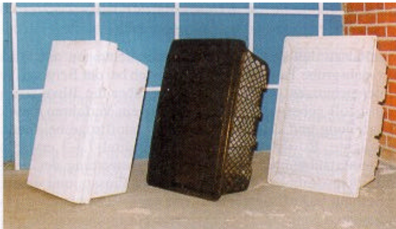
Figure 6.2a: Water troughs made out of different materials Left - Styropor, Centre - Polyvinyl chloride, Right - Polystyrol
