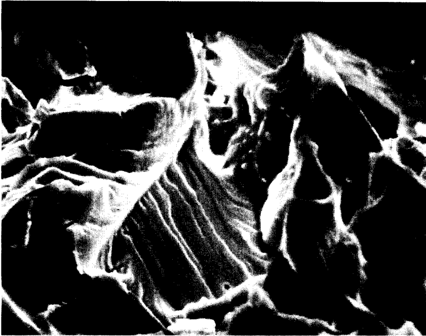
Fig. 7. Brittle cleavage fracture in embrittled samples of CZ109 brass.
