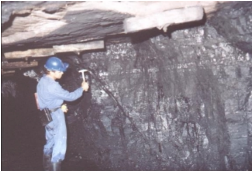
Figure 2-4 Through-going joint in a pillar at the Klip River case study
