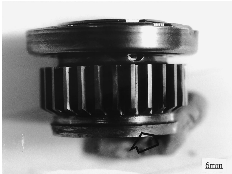
Fig. 8. Fractured PT6A-114 first stage reduction carrier (arrow indicates fracture surface).
