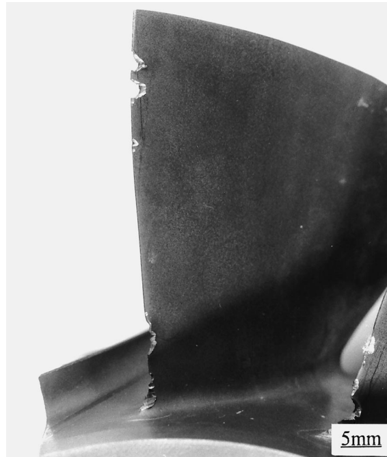
Fig. 1. Foreign object damage to PT6-65AR first stage compressor blades.
