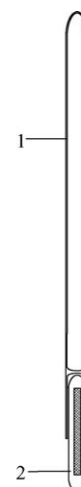
Fig. 2. Construction of the basic stirring rod. (1) Thin-walled glass tube and (2) Teflon-coated magnetic stir bar which is a sliding fit into the bottom of the glass tube.
