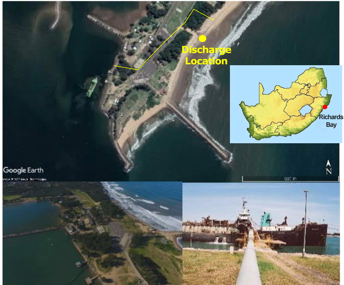
Aerial view of the existing dredge spoil disposal operations discharging spoil onto the Alkanstrand Beach. Source: van Ballegooyen, R.C. and G. Jacobs (2020) Nseleni Independent Floating Power Plant (NIFPP) and associated infrastructure, Port of Richards Bay, KwaZulu-Natal: Dredging and Dredge Spoil Disposal Modelling Study. WSP Report 431 001 376-R01, 112 pp.
