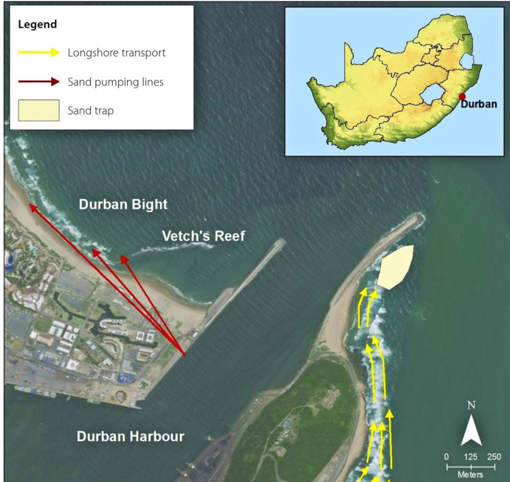
Image of Durban Harbour, indicating the locations of the sand trap, harbour entrance and Durban Bight, with (inset) a map of southern Africa showing the location of Durban. Source: Rautenbach, C. and A.K. Theron (2018) Study of the Durban Bight shoreline evolution under schematised climate change and sand-bypassing scenarios
