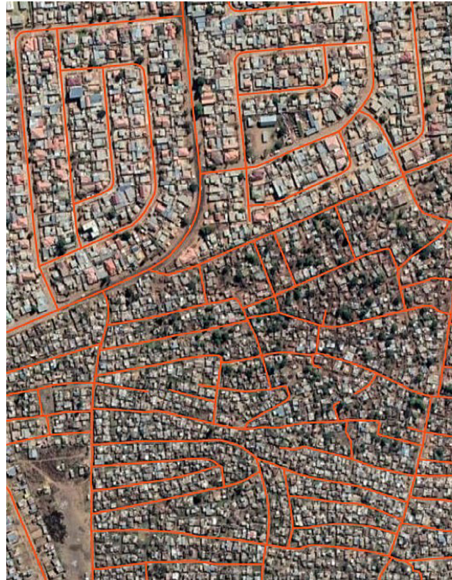
Fig. 1. Satellite imagery of formal and informal roads in Mamelodi township, South Africa. The formal roads in the upper part of the image have a more planned structure with larger gaps between roads. The informal roads in the lower part of the image have a less planned, more organic structure and smaller spaces between roads.
