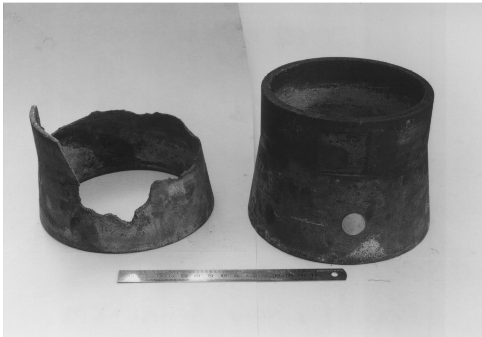
Fig. 8. Cast-iron sleeves showing severe corrosion and wear (left-hand side).
