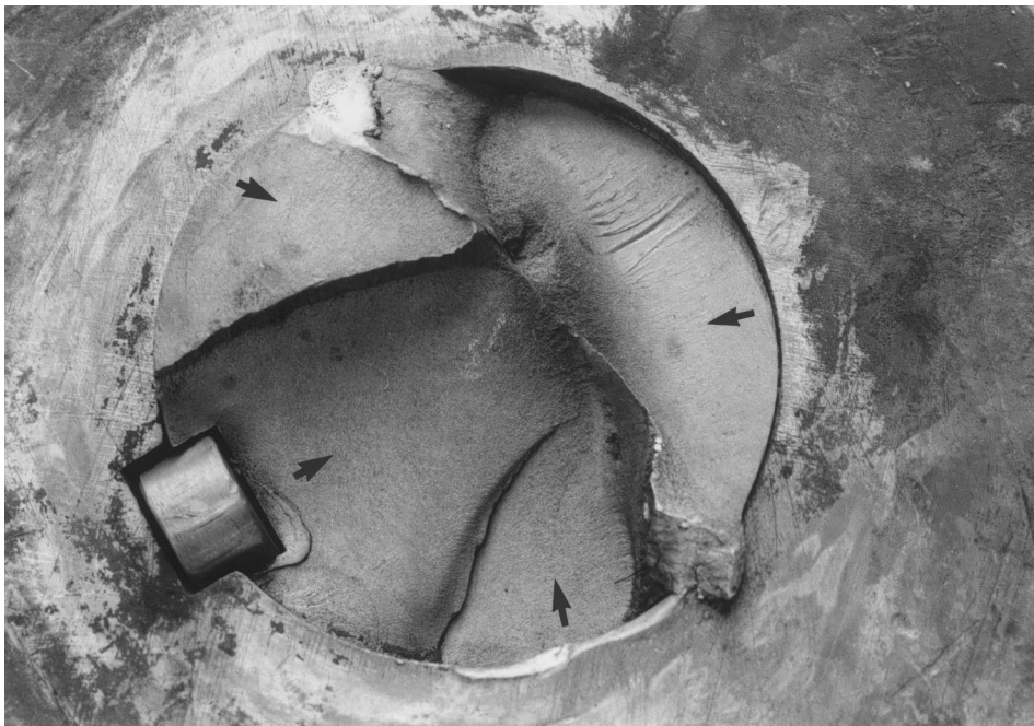
Fig. 7. Fatigue failure with multiple initiation. The arrows point to fatigue crack planes.
