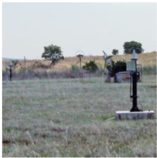
Egnos: ESA, EC and EUROCONTROL satellite-based augmentation system; supplements GPS, GLONASS and Galileo systems by reporting on signal reliability and accuracy. HBK is an EGNOS ground station (2003).
