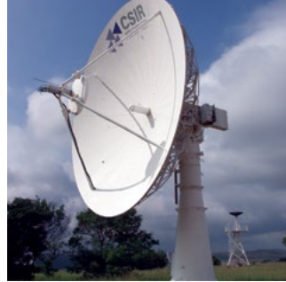
HBK-5: 10 m S- and X-band antenna with a 10°/sec slew rate, programme and auto-tracking. Installed in 1988 to provide TOSS, launch support and download Earth observation data. Known as LSX.
