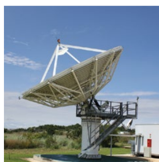
HBK-15: 9 m Ku-band antenna with a 5°/sec slew rate, programme and auto-tracking. Installed in 2006 and used for housekeeping of satellite constellations.
