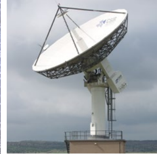
HBK-8: 13.2 m Ka-band antenna with a 2°/sec slew rate, programme and auto-tracking. Installed in 2001 to provide TOSS and IOT support.
