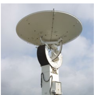
HBK-9: 5.4 m X-band antenna with a 3°/sec slew rate, programme and auto-tracking. Installed in 2002 and used to download Earth observation data.
