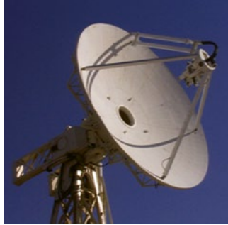
HBK-4: 6.1 m S-band uplink antenna with a 10°/sec slew rate, slaved to receive antenna systems, either HBK-2 or HBK-5. Installed in 1982. Known as S.A.T.A.N.
