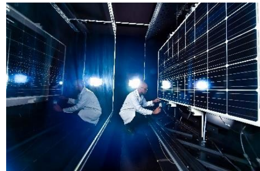
Fig. 3. PV module mounted inside the sun simulator thermal chamber with glass door.
