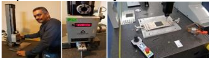
Fig.4 Thickness measurement with electronic height gage and distortion measurement with CMM
