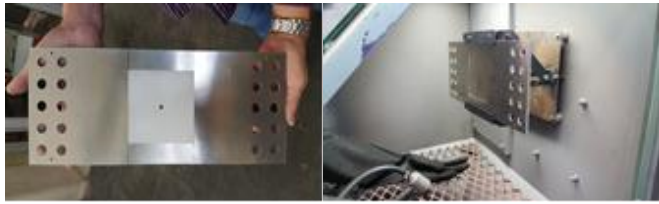
Fig.2 Surface preparation with sand blasting method
