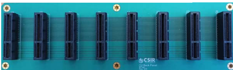
Fig 6: Control Unit backplane using PCIe connectors.
