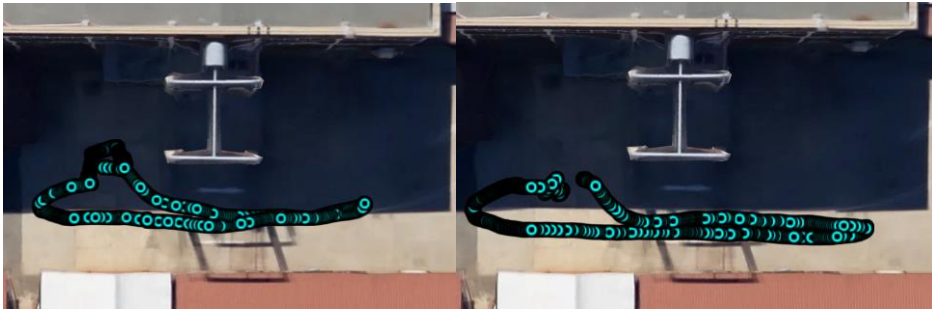
Fig. 9. Left, GPS data with no Base Station, Right, GPS data with Base Station
