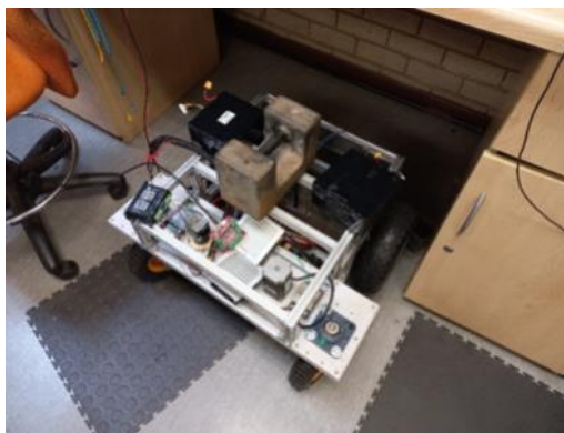
Fig. 2. Voyager version 0 undergoing active steering tests.
