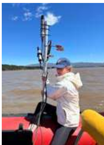
In-air measurements are taken over the water body by the NASA aircraft (left), while simultaneous radiometric measurements and water samples are collected by boat (middle), which are subsequently analysed in the lab (right).
