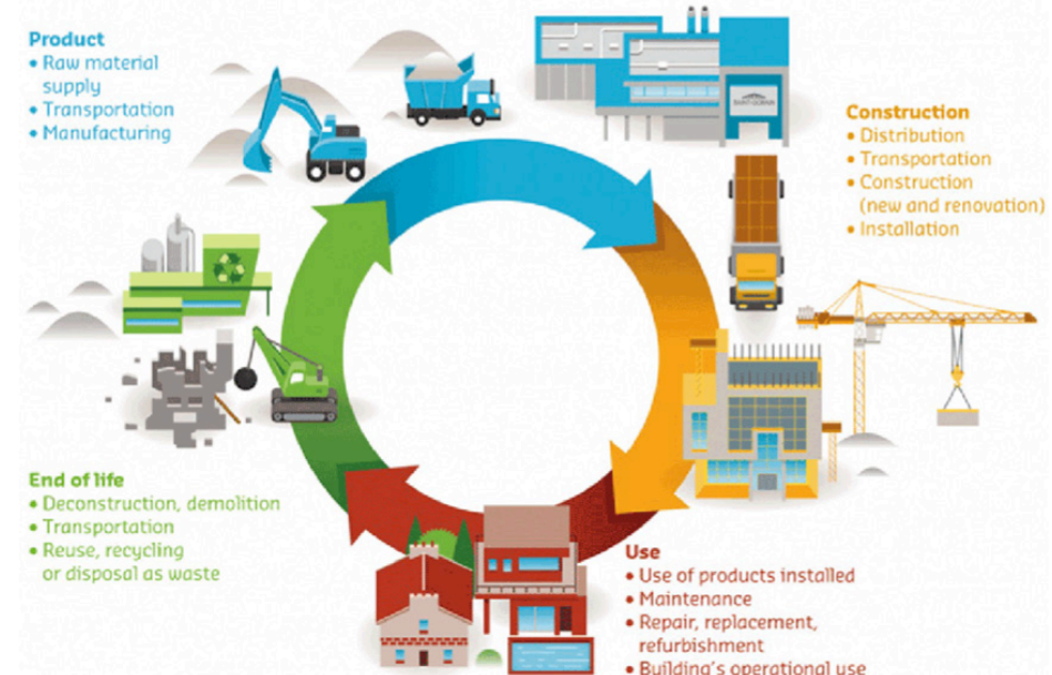
Figure 2.1: Life cycle stages of construction product (Saint-Gobain, 2017)
